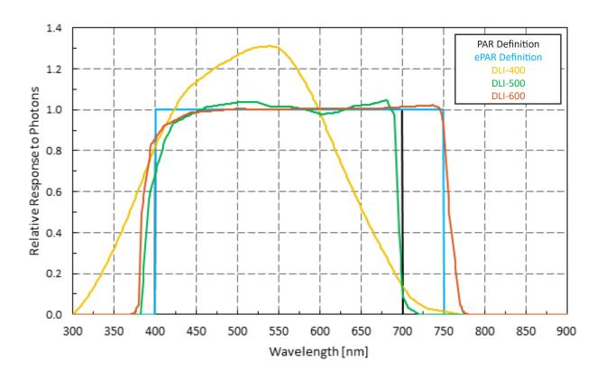
The DLI meters have a spectral range of 400 to 700 nm PAR (DLI-400 and DLI-500) and 400 to 750 nm ePAR (DLI-600). The spectral responses of DLI-400, DLI-500, and DLI-600 can be seen in the graph above. Mean spectral
