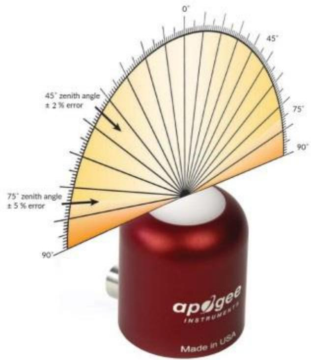
Directional, or cosine, response is defined as the measurement error at a specific angle of radiation incidence. Directional error for Apogee S2 series red - far-red sensors is approximately  $\pm 2\%$  and  $\pm 5\%$  at solar zenith angles of  $45^\circ$  and  $75^\circ$ , respectively.
