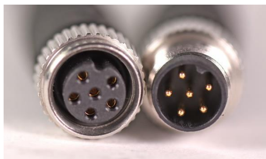
A reference notch inside the connector ensures proper alignment before tightening.
